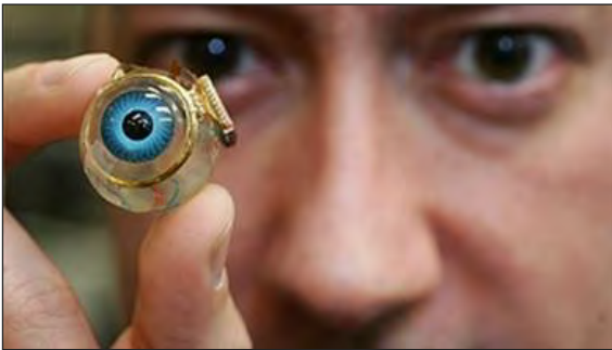
Argus II retinal prosthesis is surgically implanted in and around the eye. (Actual prosthesis pictured)
